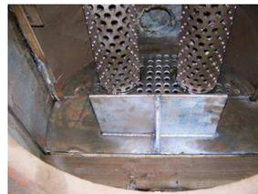
These modifications tripled the life of the cooler and similar results were attained on subsequent modifications. This proved, conclusively, that the hypotheses were indeed the main root causes of the failures.
