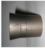
Then, to verify the above hypotheses, cones were installed at the entrance to the first-pass tubes
